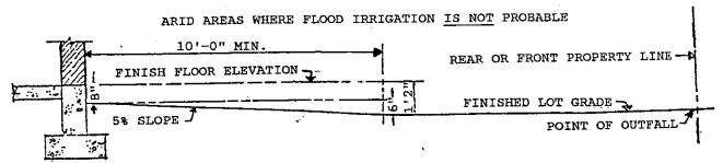
SLOPE DOWNWARD FROM WALLS AND FOUNDATION OF BUILDING AT 5/8" PER FOOT (5%) FOR AT LEAST 10 FEET AND THEN LEVEL OFF IN ORDER TO RETAIN AS MUCH WATER AS POSSIBLE ON LOT.
